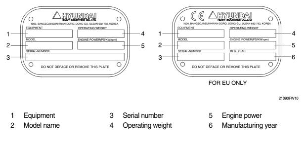
\* The machine serial number assigned to this particular machine and should be used when requesting information or ordering service parts for this machine from your authorized HYUNDAI dealer. The machine serial number is also stamped on the frame.
